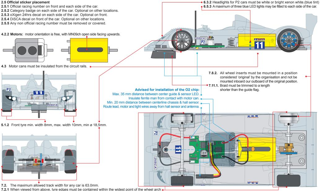
7.2.2 Body shell maximum sizes stated and tolerances stated in 2.2 still apply.
